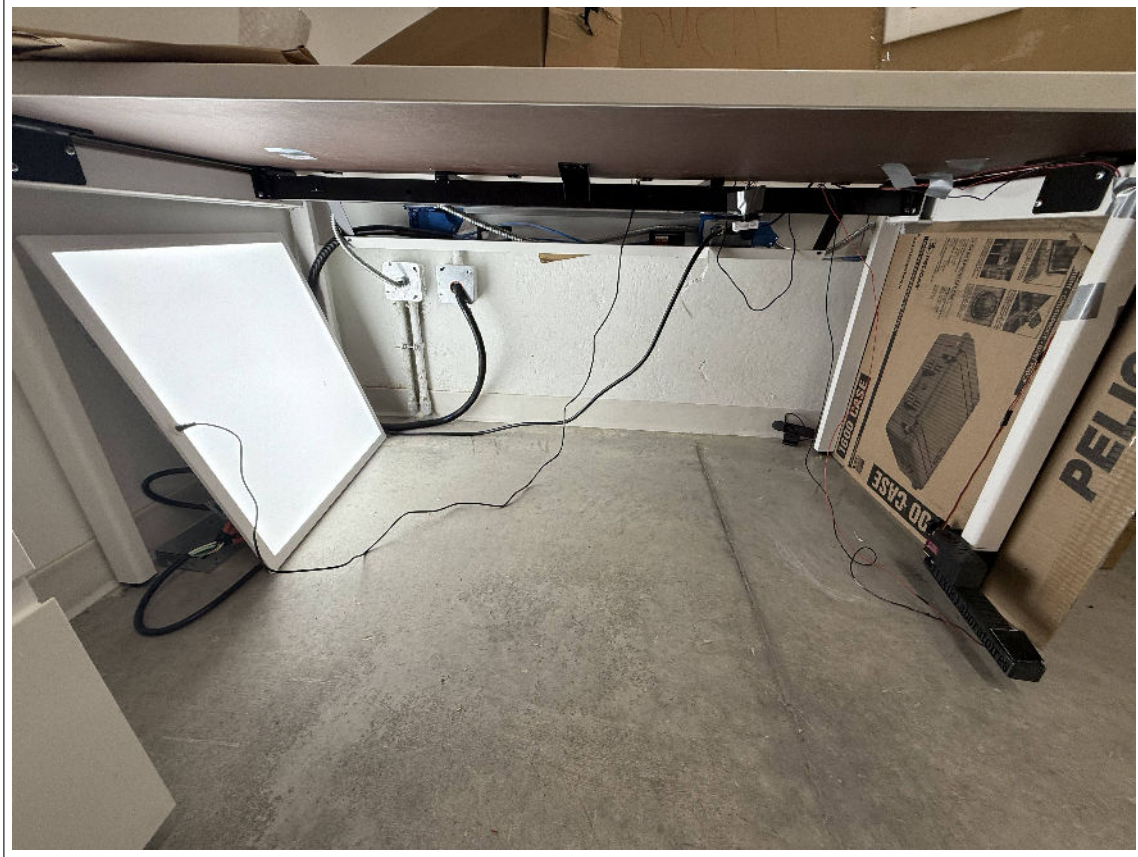
Figure 2: Photograph of the physical experimental setup used during testing, including the sensor mounting position, LED panel, and actuator based stimulus system. The isolation panels used during testing are not shown for visibility.
